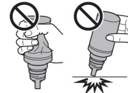
**Note:** Ink flows into the tank and stops automatically when the ink tank is filled to the upper line. If ink does not flow from the bottle, lift and reinsert the bottle.
