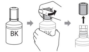
**Caution:** Do not shake or squeeze the ink bottle. Do not touch the top of the ink bottle after its cap is removed.
