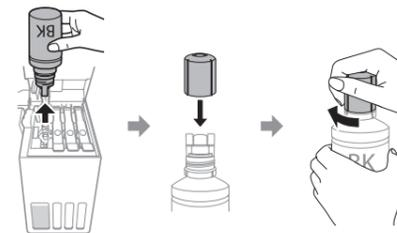
**Note:** Do not leave the ink bottle inserted; otherwise the bottle may be damaged or ink may leak.
