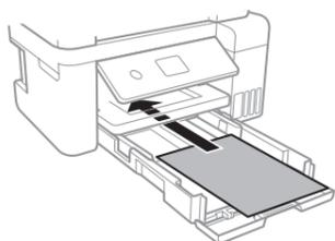
**Note:** Make sure the paper is loaded against the front edge guide and not sticking out from the end of the cassette.
