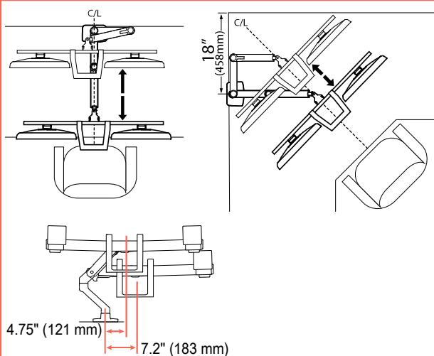
**EN** NOTE: Determine if arm will typically collapse to the left or right before installation.
