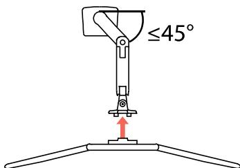
**EN** NOTE: Arm extension should be at a 45 angle or less when attaching crossbar.
