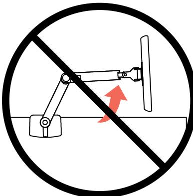
**EN** CAUTION: DO NOT rotate monitor past rear edge of desk. Doing so will create an unstable situation and may cause equipment damage or personal injury.
