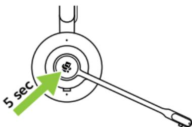
2. Press and hold the **Call** button on the headset for 4 seconds until the LED flashes blue and you hear a tone. The headset is now ready to pair.
