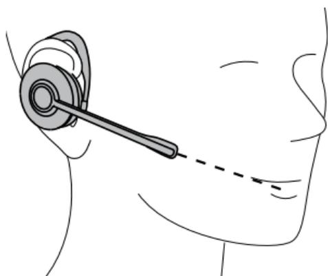
4. Ensure the earhook is fitted to the back of your ear without a gap. Adjust the earhook if necessary.
