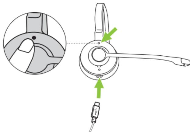
3. The headset can now be selected as an audio playback device on the computer. When the headset is connected with the USB cable, call controls and the Busylight on the headset are not supported.
