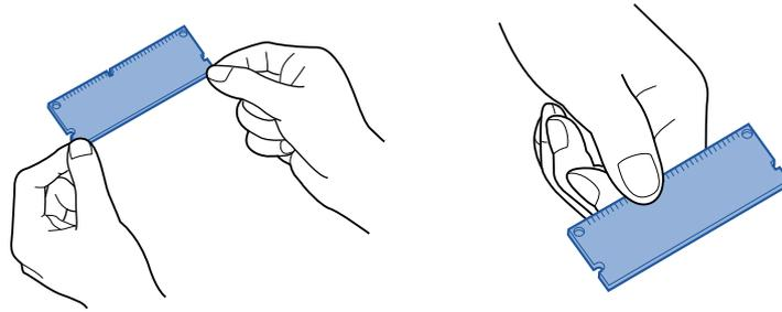
Electrostatic charge that builds up in the body through contact with clothing, carpeting, and other sources is a major enemy of chip memory. To protect memory from damage caused by electrostatic charge, touch a water tap or some metal object to discharge it from your body before loading the expansion memory. If possible, you should wear an anti-static wristband or take other anti-static measures.
