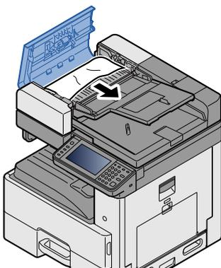
**3** Open Reverse Unit C and remove any jammed paper.
