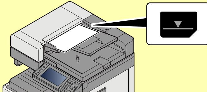
**Ensure that loaded originals do not exceed the level indicator. Exceeding the maximum level may cause the originals to jam.**
