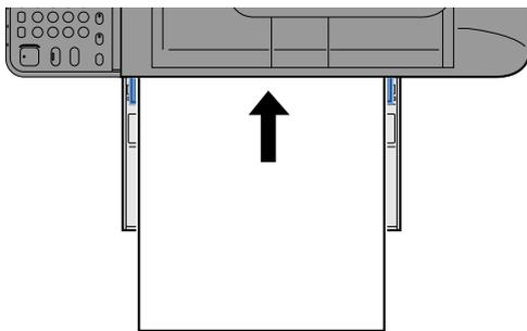
Insert the paper along the paper width guides into the tray until it stops.
